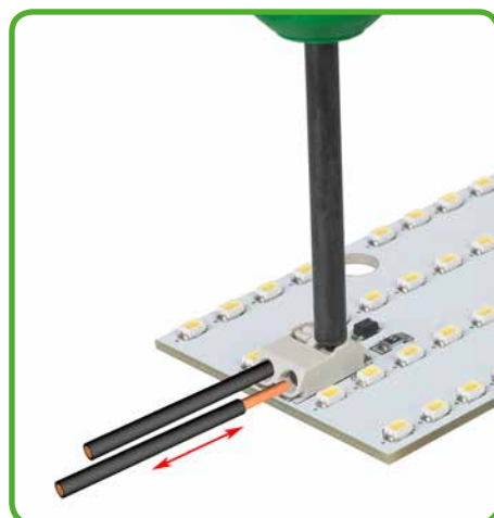
Inserting/removing fine-stranded conductors by lightly pressing on push-button (e.g., using a 206-861 operating tool).
