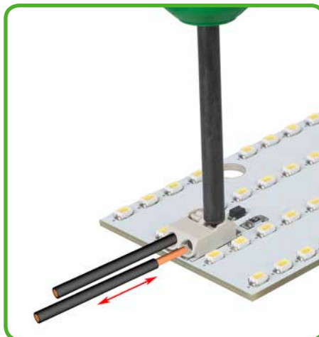
Inserting/removing fine-stranded conductors by lightly pressing on push-button (e.g., using a 206-860 operating tool).
