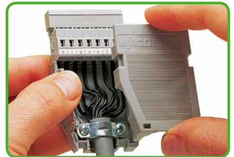
Snapping on a strain relief housing, demonstrated with a male connector. Cable exits lengthwise. Strain relief by cable clamp.
