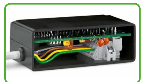
Angled female connector mounted within a housing. A male header with straight pins is used for horizontal PCB mounting in narrow housings.
