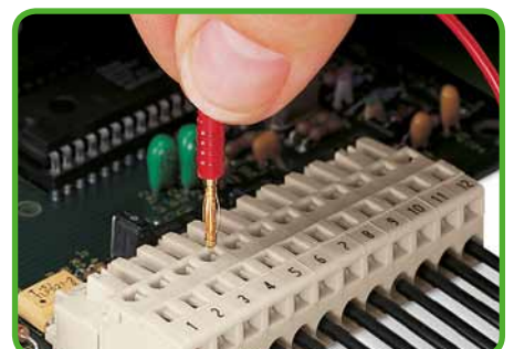
Testing – female connector with CAGE CLAMP®. Vertical insertion of Ø 2 mm and Ø 2.3 mm test plugs.
