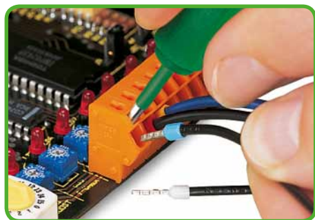
The blade dimensions of the above-listed operating tools are ideal for operating both PCB terminal blocks and MCS connectors.
