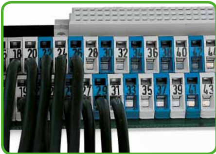
Terminal strips placed behind each other save space – staggering them by half the pin spacing simplifies subsequent wiring of the first row.
