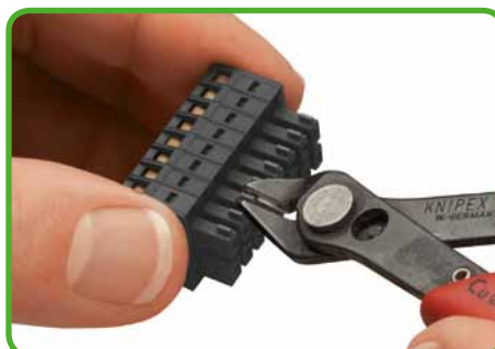
Coding a female connector.
