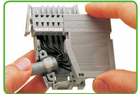
Snapping on the strain relief housing, demonstrated with a female connector with locking levers. Cable exits laterally. Strain relief by cable tie (up to a width of 4 mm).
