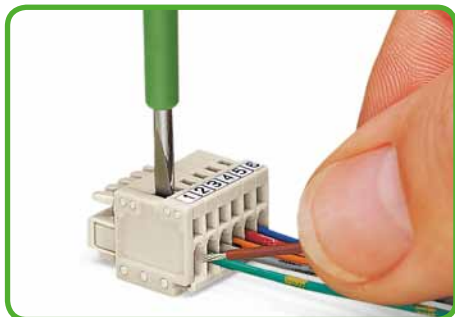
Inserting conductor via (2.5 x 0.4) mm screwdriver. Actuation perpendicular to conductor entry.
