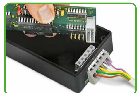
Angled female connector used as through-panel connector. Termination ports and operating slots are located outside the housing. Panel thickness up to 2 mm/0.079 in. Picture shows 5 mm/0.197 in pin spacing.
