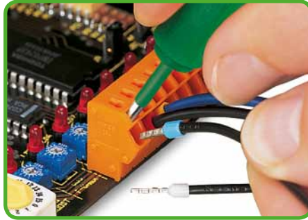
Inserting/removing ferruled conductor.
