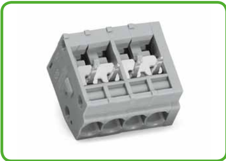
The 805 Series terminal strips provide "internal commoning" to meet requirements for not routing the ground (earth) conductor over the board. This enables custom terminal strips to be commoned and marked at the factory upon request.
