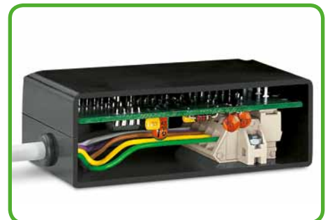
Angled female connector and male header with straight solder pins used for horizontal PCB mounting in narrow housings.
