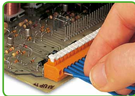
Inserting solid conductor via push-in termination.
