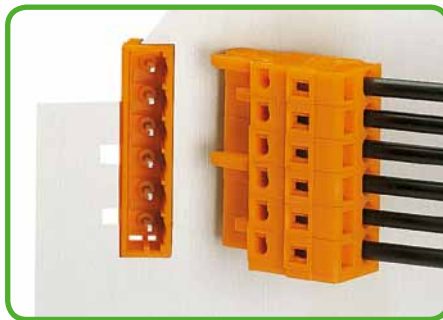
Panel feedthrough male header in small cutout. Coding with coding holes. Leave the coding finger(s) on female connector in position(s) of coding openings. Break off remaining fingers.
