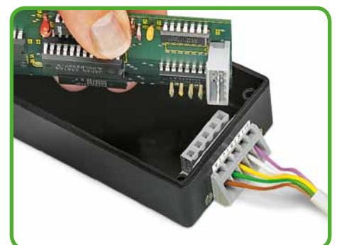
Angled female connector used as through-panel connector. Conductor entry and operation holes outside the housing. Panel thickness up to 2 mm/0.079 in.
