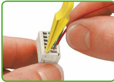
Inserting conductor via 233-331 operating tool. Operation parallel to conductor termination.
