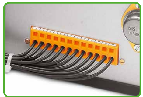
PCB female connector with fixing flanges used as through-panel connector for external wiring.
