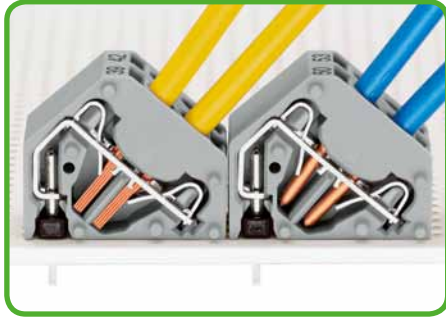
Inserting solid conductors via push-in termination. Inserting/removing fine-stranded conductors: Open clamping unit using a screwdriver and insert stripped conductor until it hits backstop.
