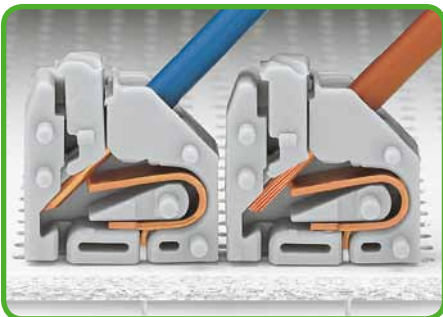
Inserting solid conductors via push-in termination. Inserting fine-stranded conductors via push-buttons, 250 Series – 3.5 mm pin spacing.
