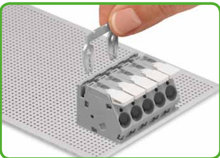
Insert the comb-style jumper bar and ...
