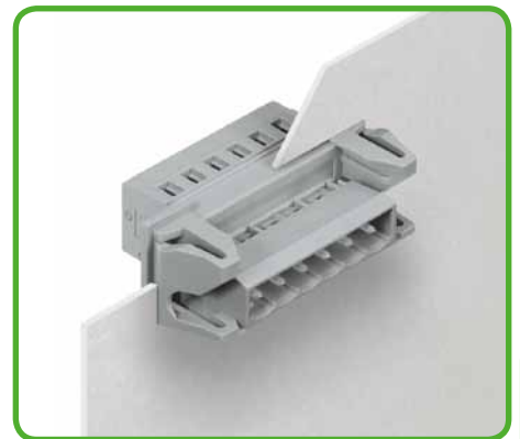
Male connectors with snap-in flanges for feedthrough applications, for 0.5 - 2.5 mm plate thickness
