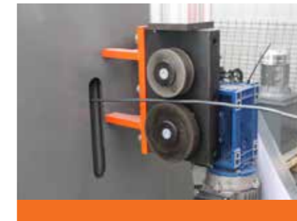
Feeding device. It helps the operator allowing the drawing of the wire from the unwinding unit to the rolling line block.
