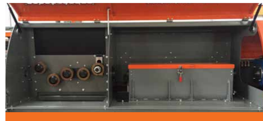
The descaling unit allows removing the calamine from the surface of the wire.
