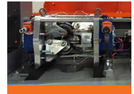
Cassette for rolling. For rolling/profiling operations. Every cassette consists of three rollers bent at 120°.
