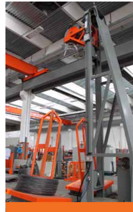
The vertical unwinding unit allows to properly unwind the wire rod.
