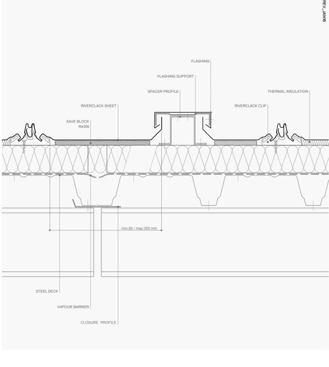
NOTES - Expansion joint has to be calculated according to actual thermal movement
