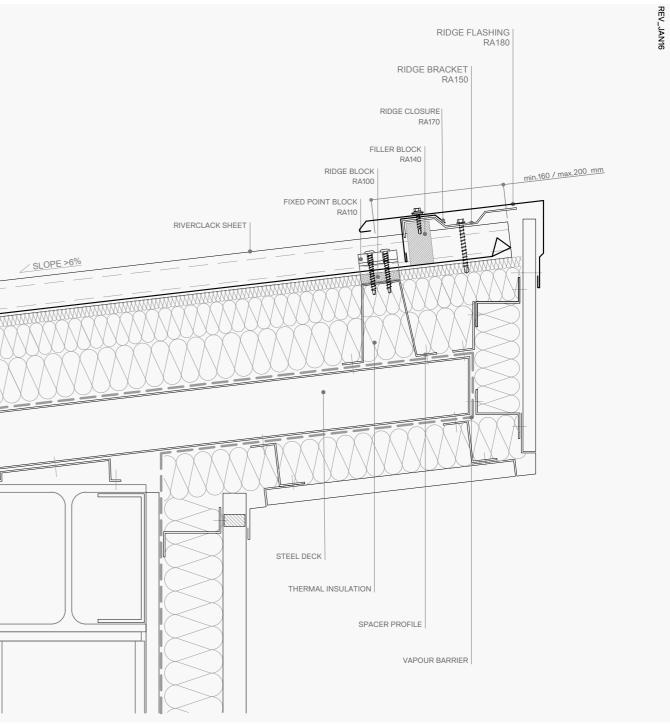
NOTES - Slope > 6% If length of sheet > 20m use item RA120 as fixed point according to instructions or use two RA110 (up to max length 40m) according to instructions
