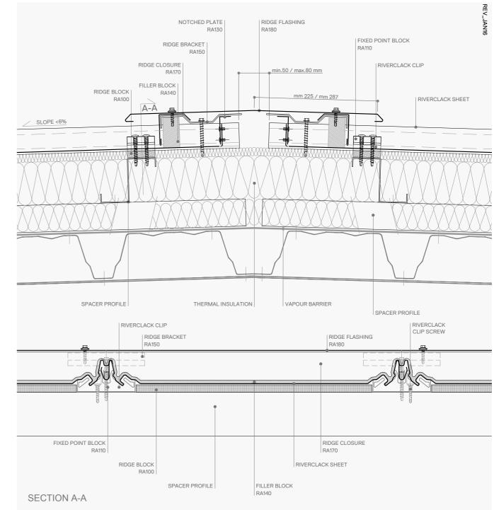
NOTES - Slope < 6% - If length of sheet > 20m use item RA120 as fixed point according to instructions or use two RA110 (up to max length 40m) according to instructions
