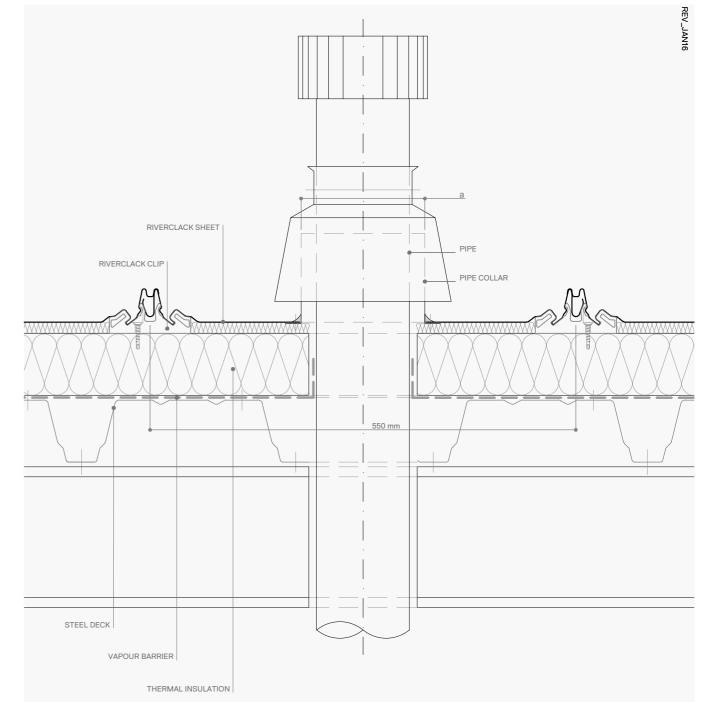
NOTES - Dimension "a" has to be calculated according to actual thermal movement
