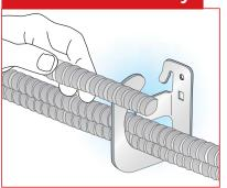
Secure MCS to structure and insert and slide cables one at a time into u-shaped slot.
