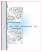
MCS can be stacked and secured with screws or nails.
