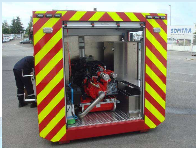
Motopompe embarquée 51,5 kW à 4600 tr/min (moteur diesel Peugeot, pompe 750 l/min) Fitted in water pump powered from one 4600 rpm 51,5 kW Peugeot diesel engine giving 750 l/min waterflow
