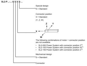
1) Collision with M12 24 V connector
