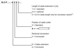
1) Connector version AVX0 refers to a 0.5 m cable extension with prefabricated connector
