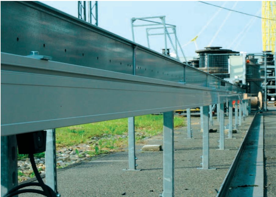
● s = 40 \text{ m} ● v = 4 \text{ m/s} ● a = 1 \text{ m/s}^2 ● m_{\text{Chain}} = 0,21 \text{ kg/m} ● m_{\text{Cable}} = 0,09 \text{ kg/m} ● Filling: 1 x CF98.05.04
