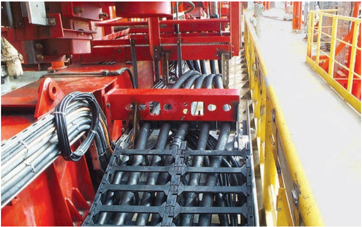
Light weight and high stability: Polymer e-chain® tames stiff hydraulic hoses
