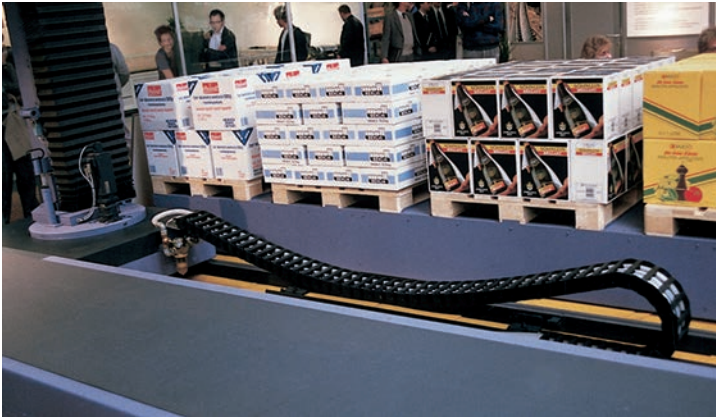
Example of unsupported permissible, FL_B
