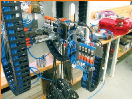
E2/000 dirt resistant e-chain®, which saves installation space - here machine tool for workpieces
