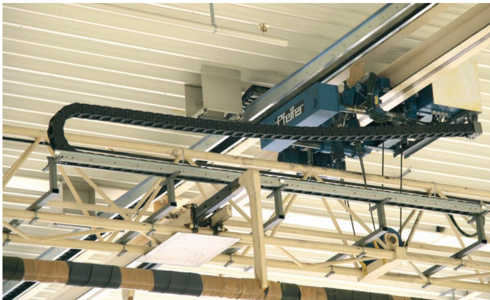
Handling unit inhouse crane - long unsupported span with an igus® E4 Series
