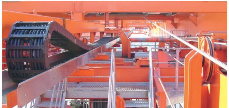
Long travel with E4/4 rol e-chain®, guided in a igus® steel guide trough
