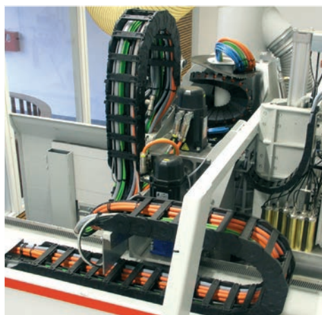
An igus® twisterband guides the energy of the 5-axis cutting heat in this wood working machine, safe and cost-effective
