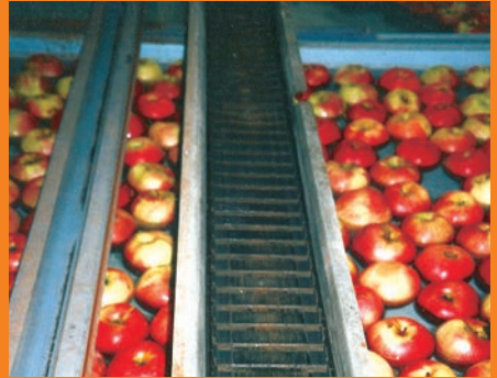
Series R68 works in an apple-sorting-machine: humidity and dirt
