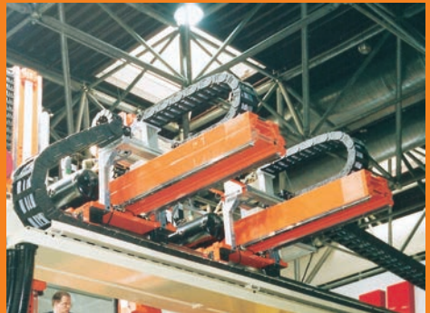
Machine tool gantry with various E4 e-chains® - fast movements and high cycle counts
