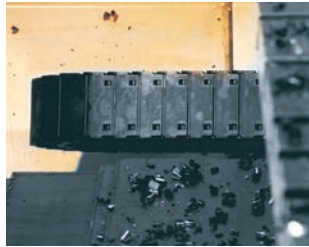
igus® e-tubes in the chip area of machine tools
