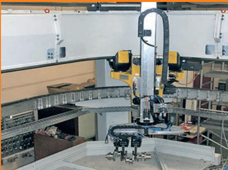
E4 e-chain® was used here in curved sections with a 45 m travel distance
