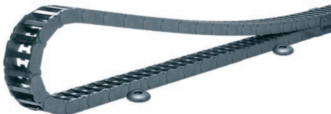
❸ autoglide glide wing and floor guide as single parts. A glide wing and floor guides every two meter completely replace a guide trough
