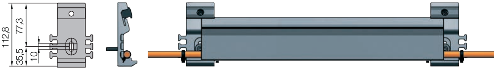
Version 01 - short trough bracket Part No. GF9.2.12 with integrated strain relief, possible ± 5 mm vertical adjustment
