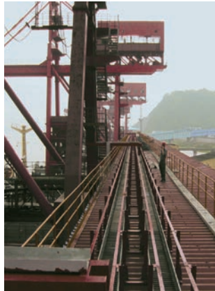
Series 4040R rol e-chain® on a coal unloading system - Travel 190 m, Speed 0.5 m/s, Fill weight 8.05 kg/m
