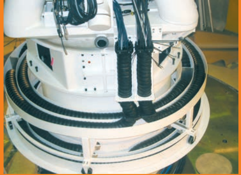
Laser measuring telescope with triflex® R. Rotary motion in both directions \leq 310^\circ possible at high speeds \leq 20 m/s
