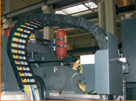
Series E4.42 in a machine tool, completely assembled with igus® chainflex® cables
