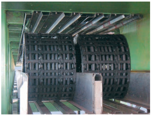
igus® System E4 with extension link at a ship loader for the coal unloading. Travel 105 m, speed 240 m/min, load 53 kg/m
