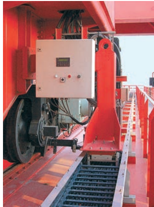
Long travels with electronics Push/Pull-force monitoring with the PPDS System
