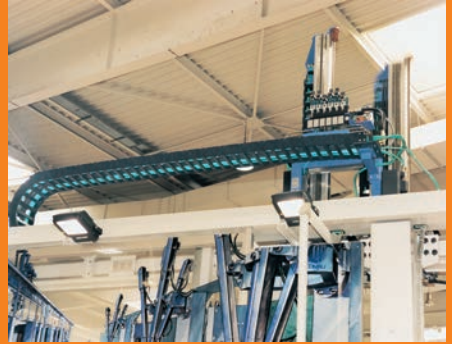
Unsupported application with harnessed e-chainsystem® E4
