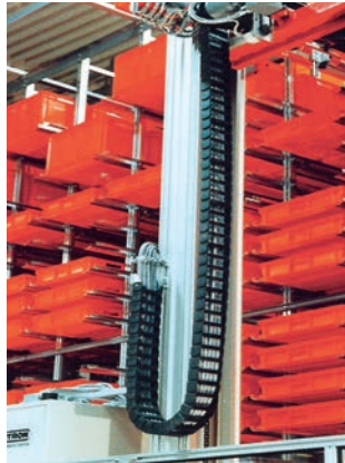
The E4.1 system is one of igus® best solutions for hanging applications
