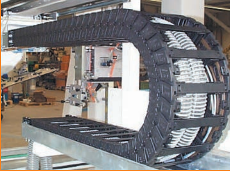
System E6 in a pick and place robot. Handles injection molded CD covers in a split second
