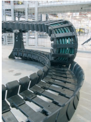
Rotary motion with new igus® generation of twisterchain®
