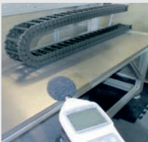
Noise level tests in igus® own acoustic laboratory
