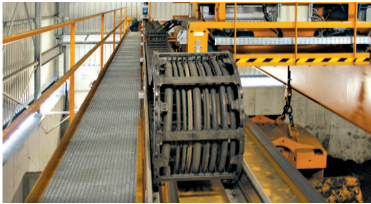
Stable guidance. Crane operating speed 80 m/min.
