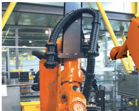
Integrated retraction spring prevents loop formation
