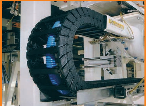
igus® System E6 - High acceleration (8 g) and ESD safety
