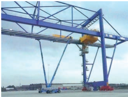
Successful application with P4.56 on a RMG crane. 130 m travel length at 150 m/min speed. Harnessed with igus® chainflex® motor-, control- and fiber optic cables
