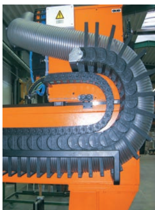
e-chain ® with extension links supports a smaller e-chain ® with electric cables
