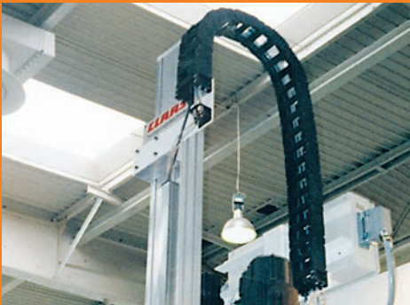
Standing application with System E4 and fixed mounting brackets
