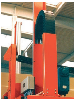
U-shaped supported e-tube for high lateral acceleration
