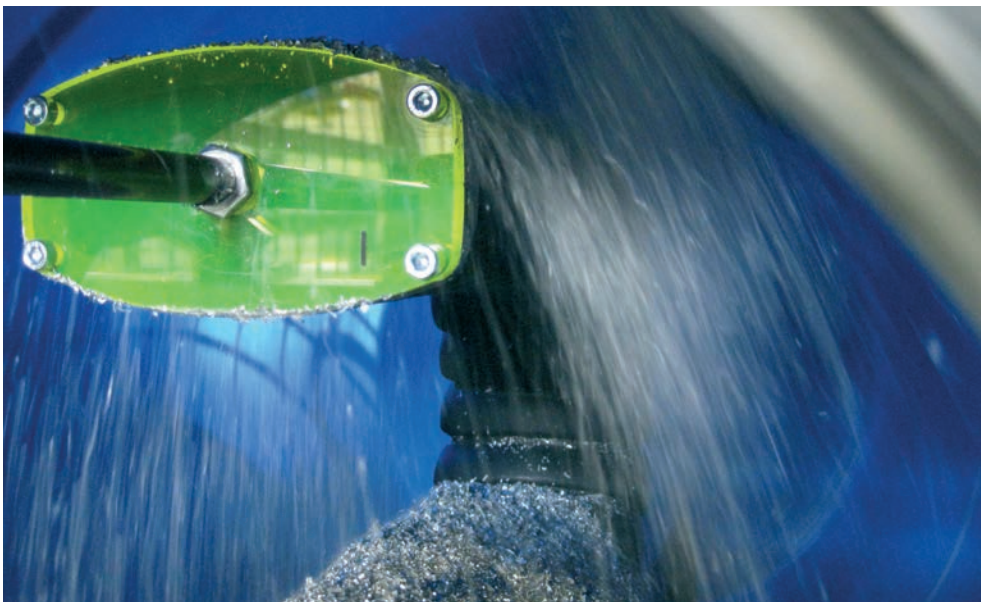
Chip tests at the igus® test-lab prove the excellent tightness of RX e-tube. Video online ► www.igus.eu/eu/RX_tested
