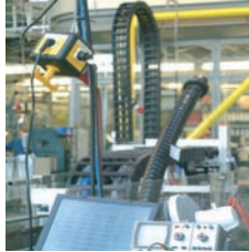
Cables are also tested for torsion properties
