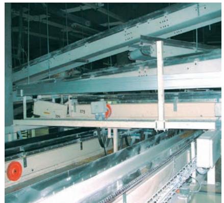
Safe energy supply also under strong dust and dirt accumulation with igus® micro flizz®
