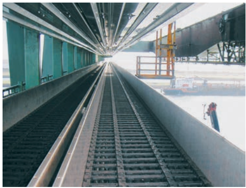
igus® System E4 with extension link at a ship loader for the coal unloading. Travel 105 m, speed 240 m/min, load 53 kg/m
