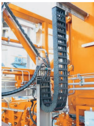
Standing applications with heights over 100 m are possible with e-chains®
