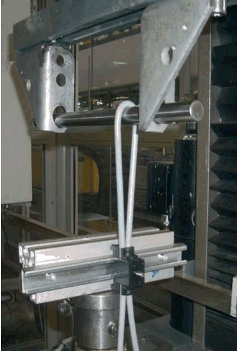
igus® tensile strength test with CFX clamps
