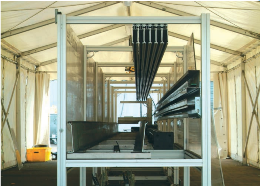
● s = 8,5 \text{ m} ● v = 4 \text{ m/s} ● a = 4 \text{ m/s}^2 ● Filling: 1x CF9.15.04 ● Running performance ca. 15.000 km without failure (issue 06.2006)
