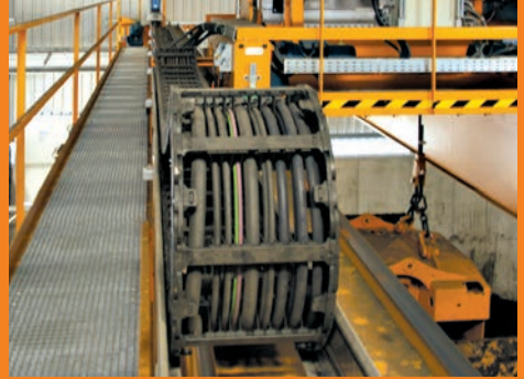
Stable guidance without oscillation. Long travel with 32 m, crane operating speed 80 m/min.
