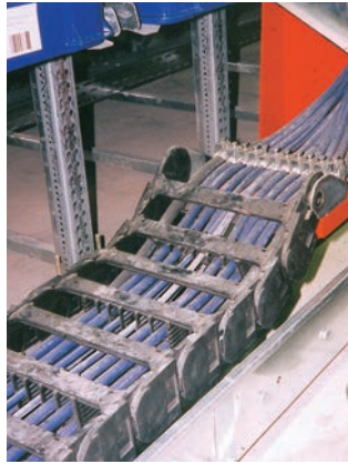
Example of lowered mounting height
