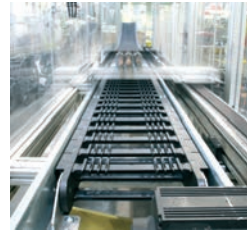
Long term wear test of P4 rol e-chains®
