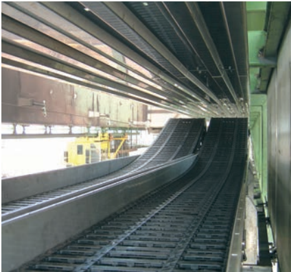
Assembled system in a ship unloading crane with 5050RHD - Travel 106 m, Speed 4 m/s, Fill weight 25 kg/m
