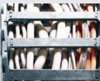
Corkscrewing: an effect of improper cable and hose placement in an e-chain®
