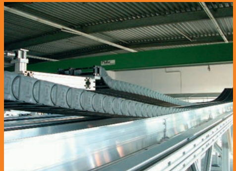
e-chain® at the mast of the shelf conveyor rolls from one aluminum guide trough to the opposite one
