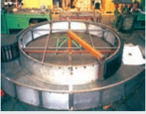
Rotary motion with RBR, diameter 6000 mm, with RBR, the inner ring rotates
