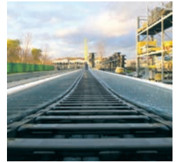
Long travel test field: 125 m travel length, speed 300 m/min
