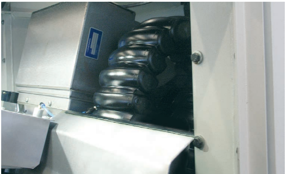
Despite the restricted installation space, the RX e-tube is used in this compact turning machine with reverse bending radius (RBR)
