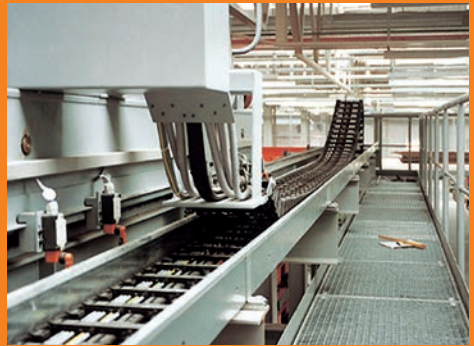
igus® steel guide trough used in a long travel robotics application
