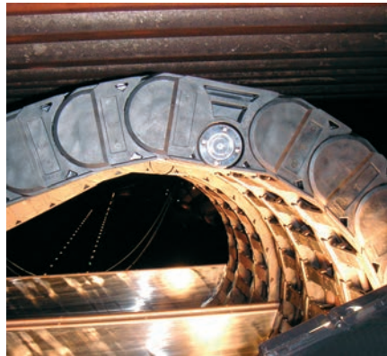
igus® e-chains® 5050RHD rol e-chain® in an igus® super-alu-trough = 75% less driving power
