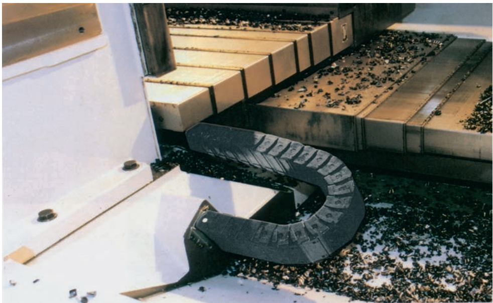
E2 e-tubes in chip-area of a tooling machine. Resistant against hot metal chips up to 850°C
