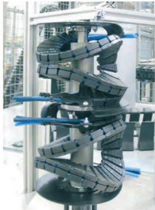
twisterband application of two systems mounted above one another
