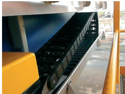
Successful application with P4.56 on a RMG crane. 130 m travel length at 150 m/min speed. Harnessed with igus® chainflex® motor-, control- and fiber optic cables
