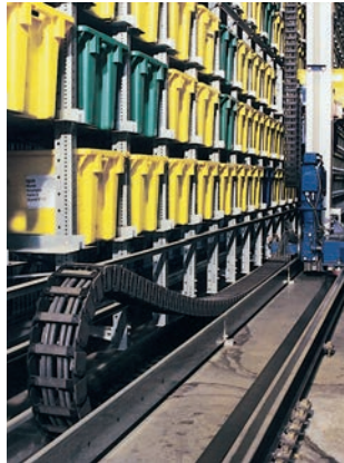
Automated storage/retrieval system with System E2 and chainflex® cables - travels up to 80 m and speed of 4.5 m/s
