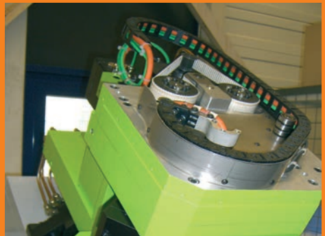
E2 mini, Series B15 - The motor spindle has a swivelling range of approx. 210^\circ
