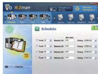
Schedule Power Management Schedule the system(s) to wake from a sleep state or turn off at a particular time
