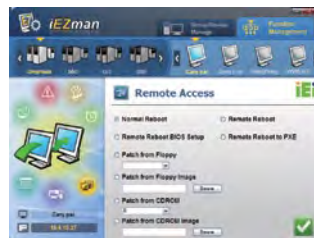
Remote Access Boot the remote PC from a local CD-ROM, floppy drive or ISO image. Or boot into the BIOS
