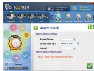
Alarm Clock Sets an alarm to wake the system even under unconnected status
