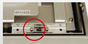
AT/ATX switch is located at the bottom right on the aluminum chassis
