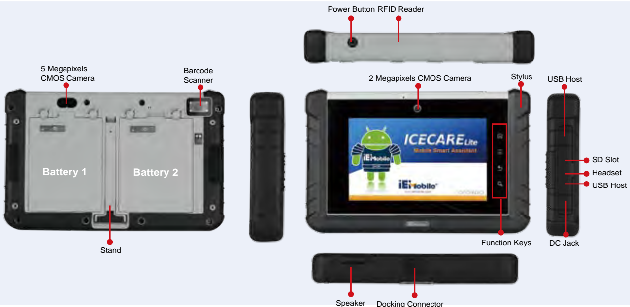
Dual hot swappable batteries
