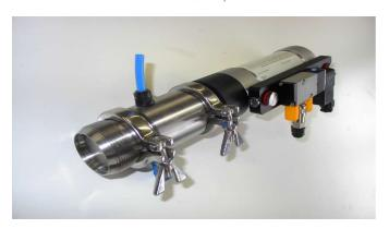
The PISTON SAMPler sampling system is designed for water sampling from pressure piping. The sampling system consists of a piston that slides into the piping profile via a fitting. During the back stroke it pulls the sample from the piping in the chamber and releases it in the sample container. The system is driven by pressured air.
