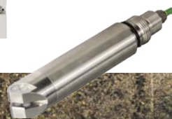
Turbidity measurement transmitter CUM 740 with CUS 65 four-beam pulsed infrared light method sensor, with automatic compensation of soiling, specifically designed to control the aeration systems.
