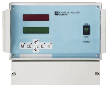
Turbidity measurement transmitter CUM 740 with CUS 65 four-beam pulsed infrared light method sensor, with automatic compensation of soiling, specifically designed to control the aeration systems.
