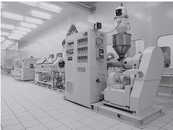
Figure B.1: Pipe extruder.
